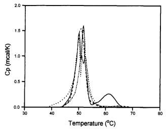
FIGURE 4: DSC profiles (excess  $C_p$  vs temperature) of LSR (4.8 mg of protein) in 1 mM CaCl<sub>2</sub> (—), 1 mM MgCl<sub>2</sub> (---), 1 mM SrCl<sub>2</sub> (…), and 1 mM BaCl<sub>2</sub> (——).
