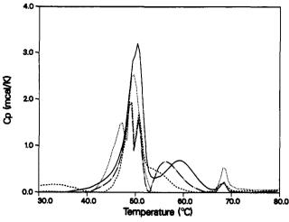
FIGURE 2: Effect of  $Ca^{2+}$  on the DSC profiles (excess  $C_p$  vs temperature) of the  $Ca^{2+}$ -ATPase of LSR. The scans (corrected for the baseline) correspond to the following free calcium concentrations (mM): 0 (...), 0.1 (---), 0.32 (---), and 1 (--).
