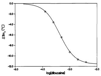
FIGURE 7: Dependence of the shift in the denaturation temperature  $(\Delta T_{\rm m2})$  on the concentration of dibucaine. The solid line represents the best fit to the Hill equation, with the parameters  $pK_d = 3.4$ , n = 1.6, and  $\Delta T_{m2}^{max}$  = -11.6 °C.
