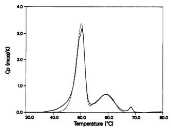
FIGURE 1: DSC profile (excess  $C_p$  vs temperature) of LSR (4.8 mg of protein) in 1 mM Ca2+ with the baseline corrected. The dotted line represents the best fit assuming two irreversible transitions with  $T_{\rm m}$ 's of 49.8 and 58.6 °C.
