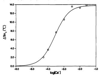
FIGURE 3: Dependence of the shift in the denaturation temperature  $(\Delta T_{\rm m2})$  on the concentration of free Ca<sup>2+</sup>. The solid line represents the best fit to the Hill equation, with the parameters p $K_{\rm d}=3.6$ , n=1.0, and  $\Delta T_{\rm max}^{\rm max}=13.8$  °C.
