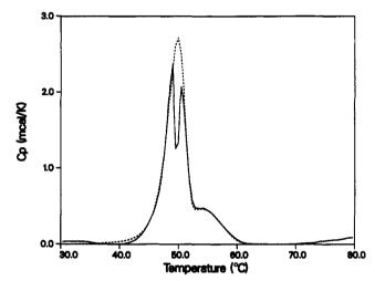
FIGURE 5: DSC profile (excess  $C_p$  vs temperature) of LSR (4.8 mg of protein) in 1 mM Ca<sup>2+</sup> and 0.5 mM dibucaine. The dotted line represents the best fit to the experimental curve, assuming two irreversible transitions with  $T_{\rm m}$ 's of 49.4 and 52.8 °C.
