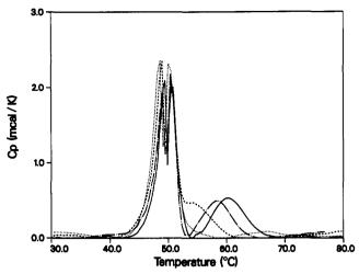
FIGURE 6: Effect of dibucaine on the DSC profiles (excess  $C_p$  vs temperature) of the Ca<sup>2+</sup>-ATPase of LSR in 1 mM Ca<sup>2+</sup>. The scans (corrected for the baseline) correspond to the following dibucaine concentrations (mM):  $0 \leftarrow 0.125 \leftarrow 0.5 \leftarrow 0.5 \leftarrow 0.5$ , and  $1 \leftarrow 0.5 \leftarrow 0.5$
